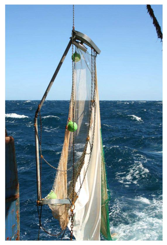
Figure 2: The beam trawl being retrieved using the recovery chain.
