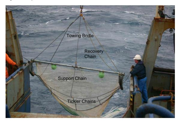
Figure 4: Lay out of the tow and tickler chains.
