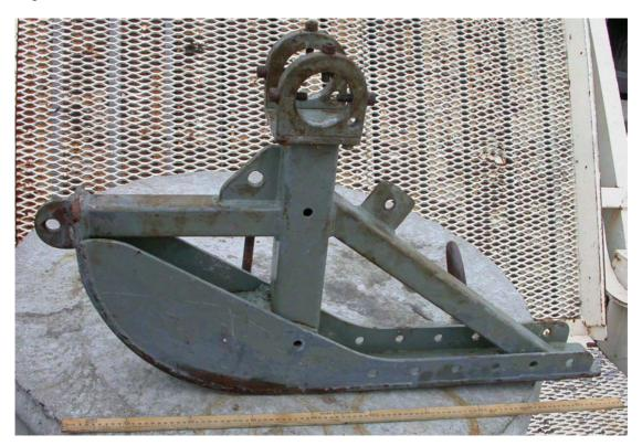
Figure 6: A side view of the beam trawl shoe.
